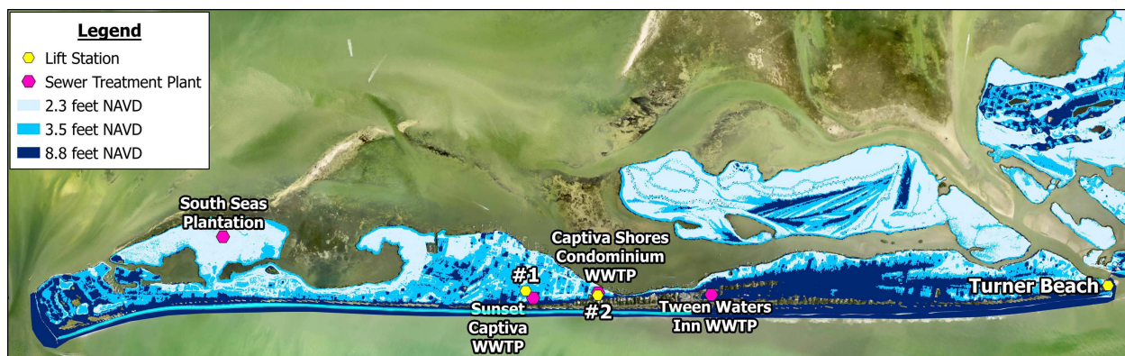
Figure 27. Wastewater Treatment Plant and Lift Station Inundation Map for Inundation Tipping Point Scenarios
