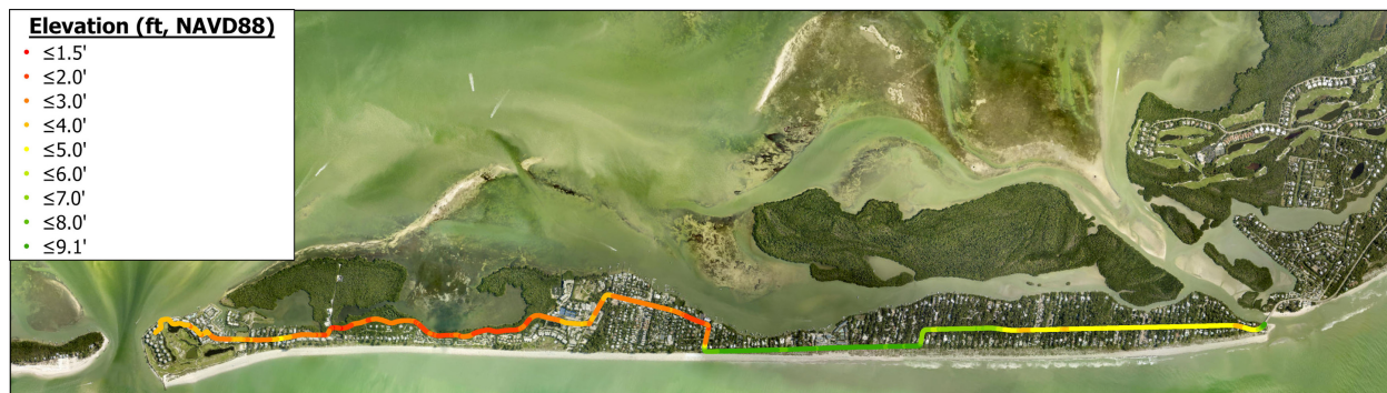
Figure 38. Captiva Evacuation Route Elevation
